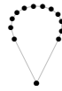
Figure 5: The PostScriptTrace() function breaks a path into a series of locations on the boundary of the path. This image shows how the curved petal shape from Table 1 can be converted into a set of points describing the outline of the petal shape.
